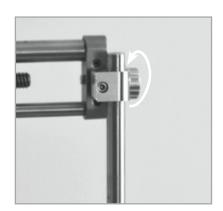
8. Connect the assembly to the frame with the screw on the stereotaxic adapter.
