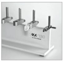
1. Fix a probe clip to the vertical pin at one end of the stand.
