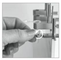
2. Open the probe clip by turning the lock screw counterclockwise.
