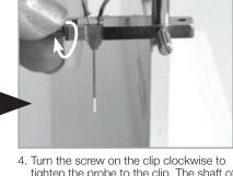
4. Turn the screw on the clip clockwise to tighten the probe to the clip. The shaft of the probe will now be vertical.
