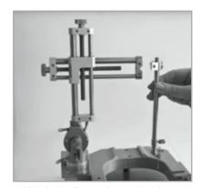
7. Unlock the clip from the stand and transfer the assembly to the manipulator of the stereotaxic frame.
